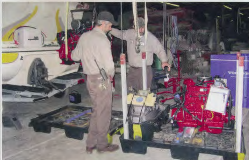
■ After running the boat with the Volvo Penta 3.0L GL, the engine was swapped out for the 3.0GXl.
