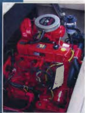
■ As a baseline, we tested Volvo's carbureted 3.0L in a Stingray 195LX bowrider.
