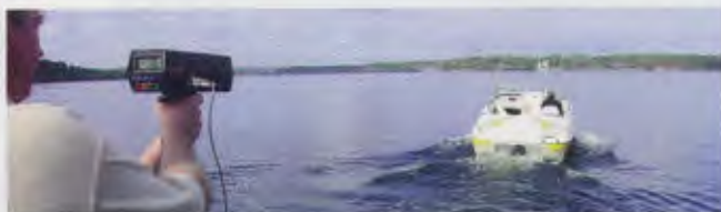
■ Stingray's sporty bowrider squeezed out nearly 2 mph with the additional 15 horsepower provided by the Volvo Penta 3.0GXi/SX sterndrive with EFI.
