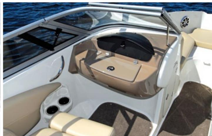
The companion console features an ice bucket below and a radio compartment above.
