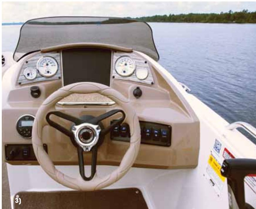
**3)** A clean helm offers a large central space for the owner's choice of electronics. Behind the wheel is a spot to place your phone next to a 12V outlet and audio input.
