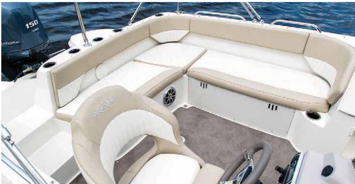
Stainless steel grab handles are considerately placed throughout the boat, as is a surplus of cup holders. Venting is provided on all large storage areas to prevent the build up of mildew and the cockpit is self-draining.
